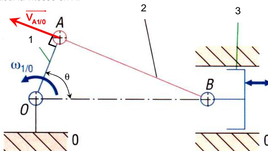
$V_A = V_{A1/0} = V_{A2/0} = \omega_{1/0} \times OA = 100 \times 0,035 = 3,5 \text{ m/s}$
